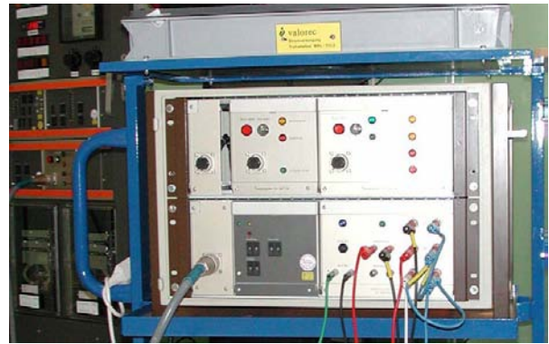
Figure 2: Test adapter for testing MC, QV and IT relays
