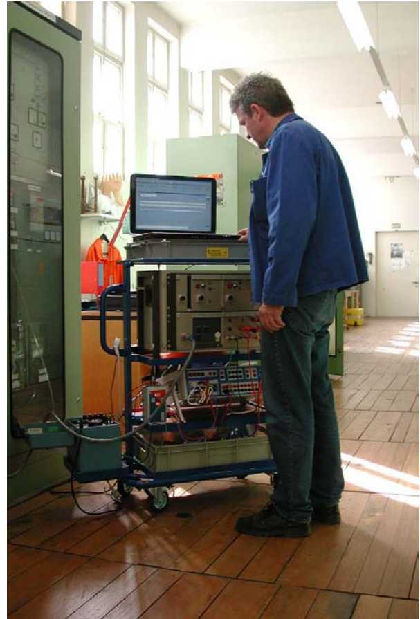
Figure 7: Automatic test MC with test adapter and CMC256/CMASB2
