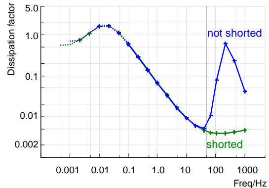
Figure 12: Dielectric response of a distribution transformer for shorted and not shorted windings
