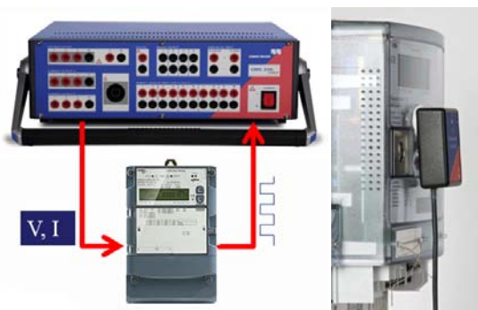
Figure 2: Meter Test set-up with new type of rubber-adhesive-fixed pick-up
