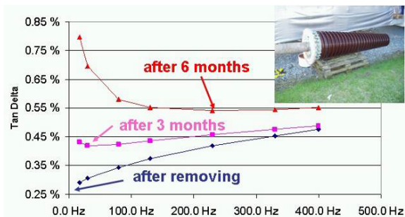
Fig. 5: Dielectric Response of a RIP bushing exposed to wet air
