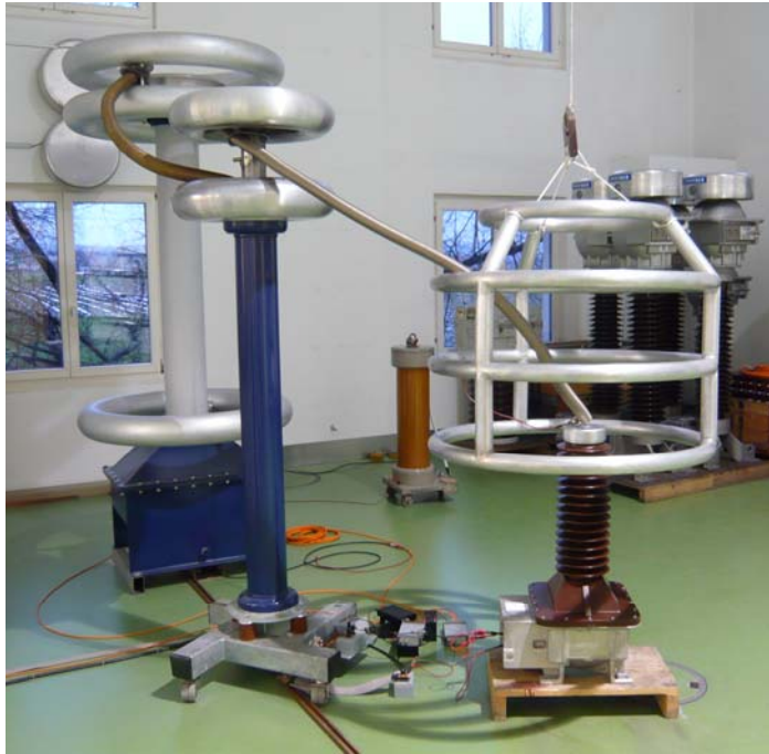
Fig 6: PD test setup according to IEC 60270 with test voltage source, coupling capacitor and test object (VT)
