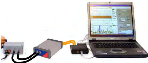
Fig. 1: MPD 600 PD measurement system (measurement impedance, acquisition unit, USB interface unit and notebook)
