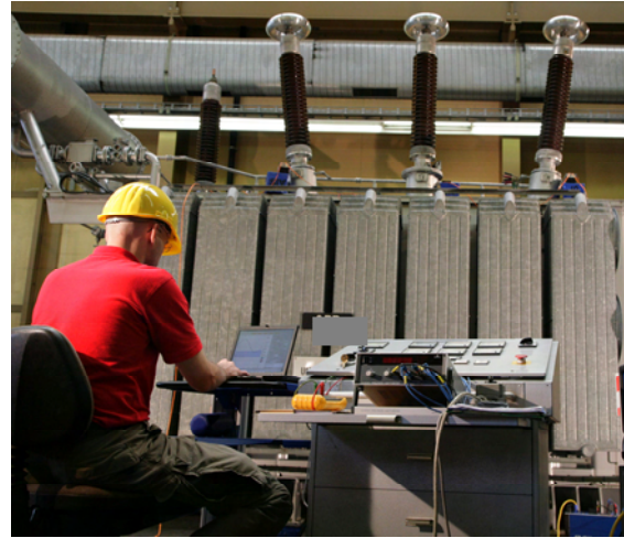
Fig. 13: PD measurement using a notebook
