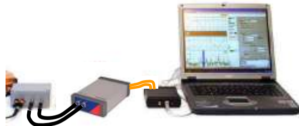
Fig. 1. MPD600 PD measuring system (measuring impedance, PD acquisition unit, optic-USB converter, notebook)
