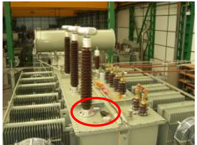
Fig. 9. PD decoupling at bushing taps
